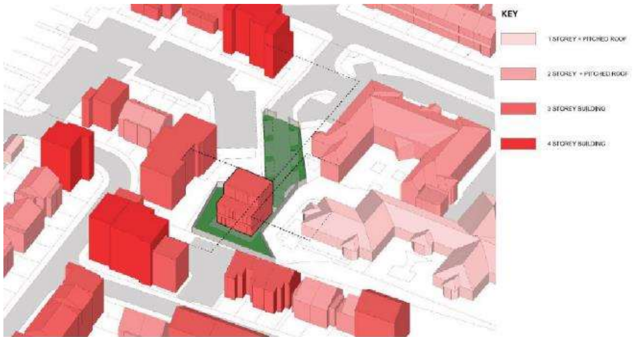
Extract from the applicants Design and Access Statement indicating the proposed buildings scale in context with adjacent buildings
